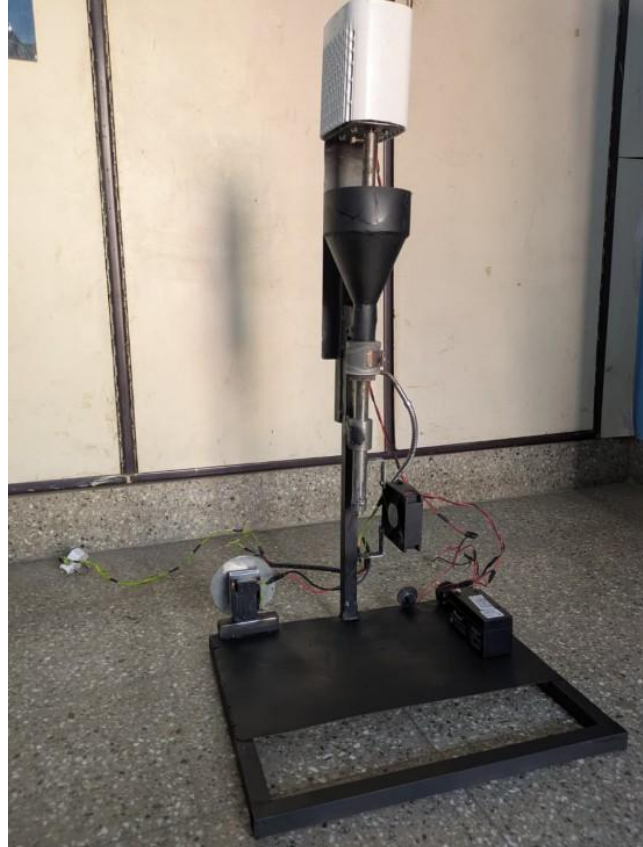
Figure 2: Fabricated Model — ISO-Left View Showing Hopper, Barrel, Motor, Cooling Fan, and Steel Base Frame
