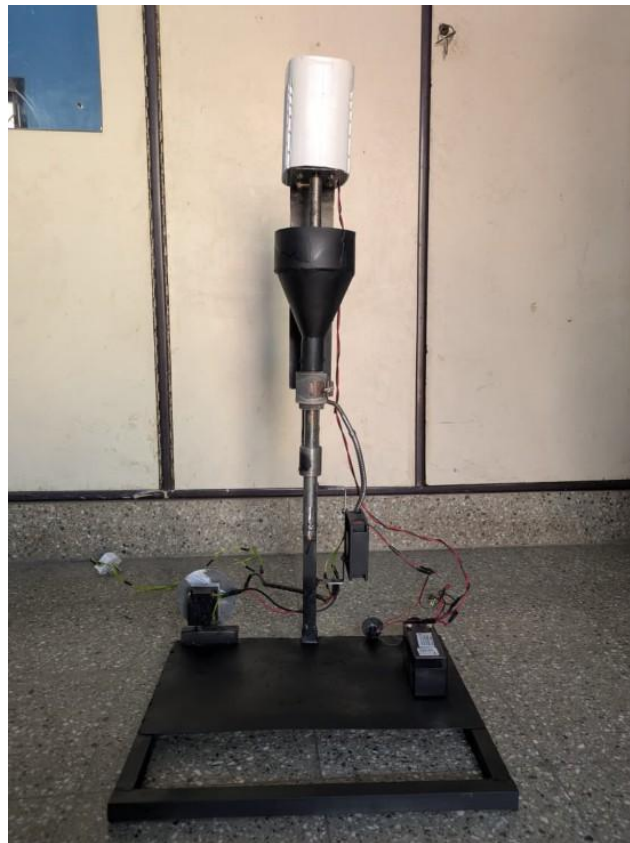
Figure 3: Fabricated Model — Front View Showing Complete Assembly of the Desktop-Scale Filament Extruder
