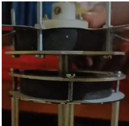
Figure 3: Magnetic Levitation Arrangement
