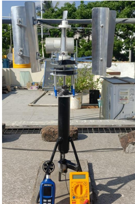
Figure 2: Fabricated magnetically levitated vertical axis wind turbine prototype
