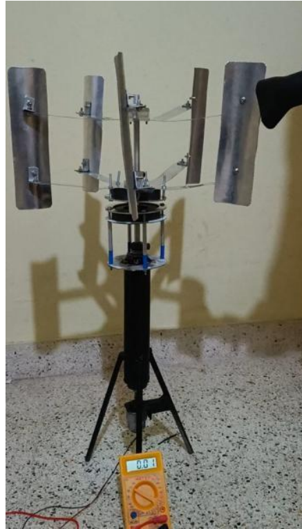
Figure 4: Experimental setup of the magnetically levitated VAWT.
