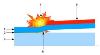
Explosive welding: 1 Flyer (cladding). 2 Resolidified zone (should be limited for welding of unique materials). 3 Target (substrate). 4 Explosion. 5 Explosive powder. 6 Plasma fly.
