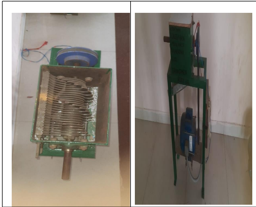
Figure 2: Sectional View of Single-Shaft Shredder Machine
