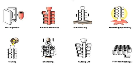
Fig.1. investment casting process (pic courtesy dly-metal.com)
