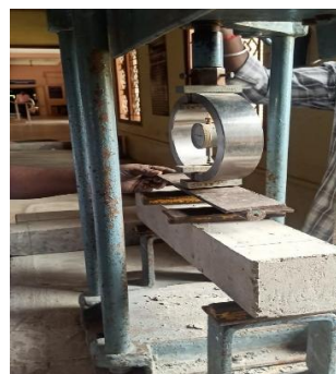
Figure 8. Flexural Test Set up
