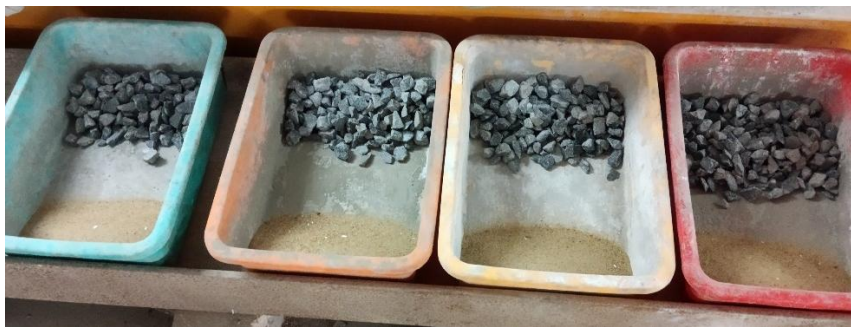
Figure 1. Coarse and Fine Aggregate Batching
