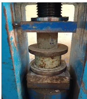
Figure 7. Compression Test Set up
